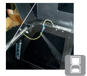
All movable machine parts are connected with the machine corpus by means of a grounding cable
