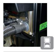
The air-ducting hoses are made of electric conductive material
