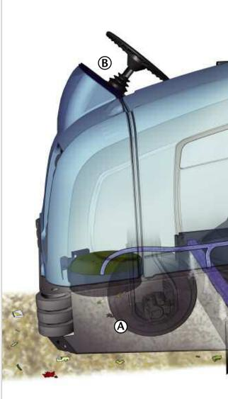
A Superior maneuverability for cleaning in tight areas with front wheel steering and high traction scrubber tires.
