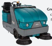
Greener alternative. High productivity cleaning of large areas with a quiet, fume-free battery version, eliminating engine exhaust.
