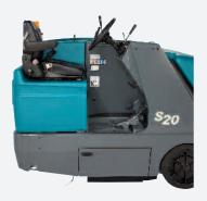
Spacious operator compartment incorporates adjustable seat, propel pedal, and steering column to customise fit.
