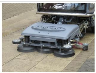
Water is suctioned with a squeegee connected to hopper via a 75 mm/3 in hose to get full suction power and great results.
